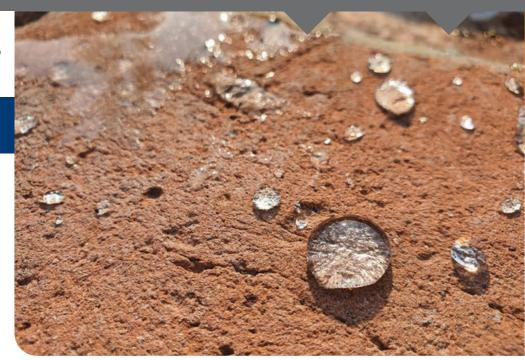
Climashield Masonry Cream is a, unique, thixotropic, water-repelling masonry protection cream which can be used on a range of building materials. Dependent on the porosity of the substrate, the effective siloxane ingredient penetrates the substrate within a short period of time (30 minutes to several hours), where it reacts to become a permanent, chemically bonded, silicone coating.
