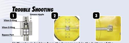
1) If water is leaking from the bypass port in the bottom of the rotary head: Inspect the viton O-Ring in the rotary head. 2)Rotary Arm doesn't spin:
