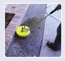
Connect to lance using q/c fittings on the lance and whirl-a-way. Ensure the M22 hose is connected properly before use.
