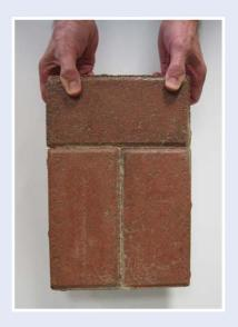
Smartseal Block Paving Sealer solidifies jointing sand between block pavers to create a strong bond.
